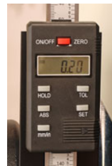
The included DRO has several functions, not the least of which is allowing ultra precise table to drum settings.
